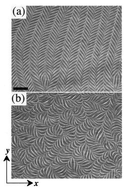
FIG. 2. One typical chevron (DFC) for  $f > f_w$  in the conduction regime. (a) A spatially double-periodic chevron pattern at V = 149.40 V and f = 3900 Hz ( $> f_w \approx 3150$  Hz), which was suddenly applied from the homogeneous Fréedericksz state ( $V_F \approx 3.92$  V). (b) A spatiotemporally chaotic pattern with local chevron structures, which was obtained from (a) after waiting 1 h. The length of the scale bar in (a) is 200  $\mu$ m.
