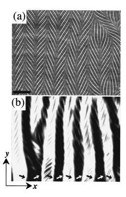
FIG. 5. Determination of the **C** director in the DFC (V = 147.7 V and f = 3900 Hz $> f_w$ ), (a) with no crossed polarizer set, and (b) under a crossed polarizer set with a 20° counterclockwise rotation to the *x* axis. The **C**-director structure for the DFC can be determined from the direction and amplitude of the rotation of the crossed polarizer set. The **C**-director structure is depicted as thin arrows in (b). The length of the scale bar in (a) is 200  $\mu$ m.
