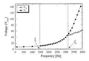
FIG. 7. Threshold  $V_w$  for the prewavy pattern in sample 3. For  $f > f_w$ ,  $V_w$  (open circles) indicates the threshold voltage for the prewavy pattern, while  $V_c$  (solid circles) indicates the critical voltage for the convection.
